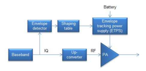
For envelope tracking PA, the envelope tracking power supply and the RF input signal should be aligned strictly in time. Even small time deviations will have substantial influence in the RF output signal, leading to the deterioration of the ACP and EVM.
