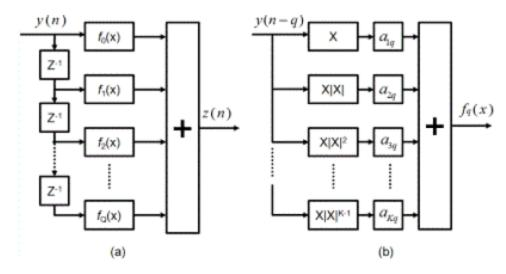
The structure of Volterra series is shown below.
