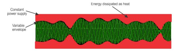
The consequence of the PA inefficiency is very practical. The smart phones will be hotter and their batteries will run out quickly; at the same time, mobile and broadcast network operators need to pay a lot for the wasted energy.
